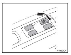
If your vehicle has this feature, the power window switches are located on the armrest on the driver's door. In addition, each passenger door has a switch for its own window. The ignition must be ON to use the power windows.
